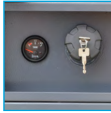
Tank hatch with key lock cap and warning light
