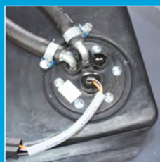
Automatic stop system due to lack of fuel
